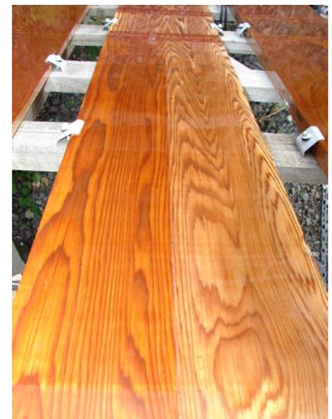
Some of the major cracks in the cedar have caused the film to rupture but the other samples look as if they had just been applied. Note excellent gloss retention – water still beads on these samples after 16 months.
