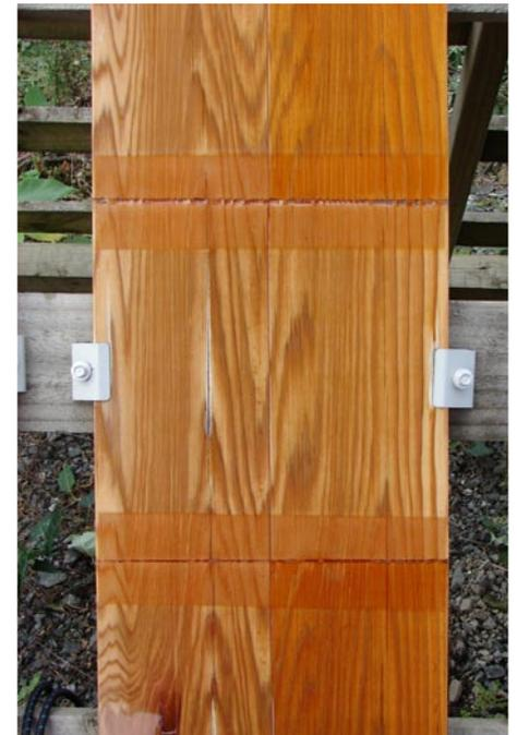
The left hand side of these panels have the clear primer and the right the coloured. The coloured primers retain colour closer to the original timber tone however the clear retains a desirable timber aesthetic. The two bands across each board are kept covered.
