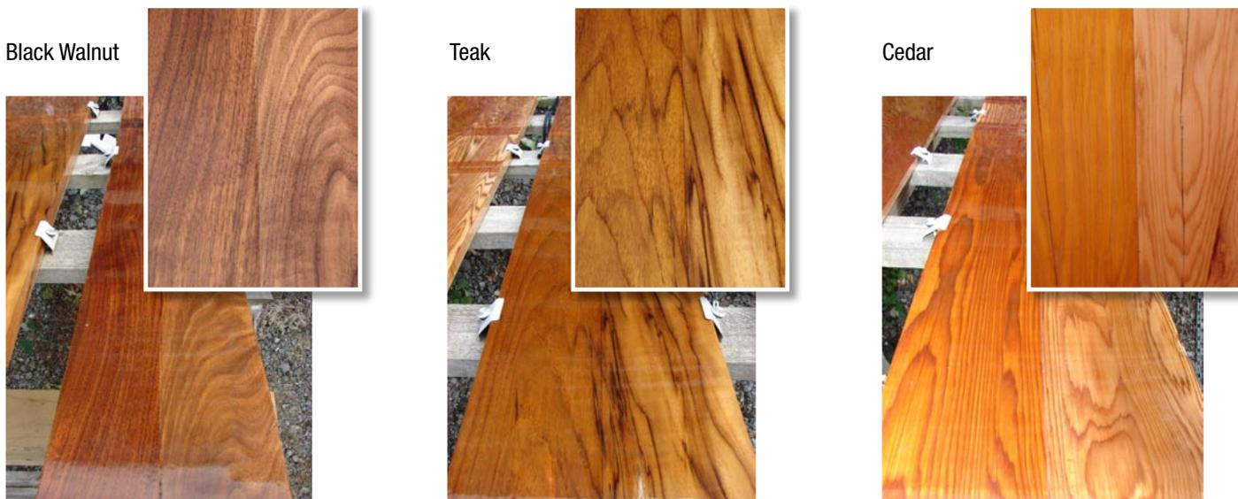
**Images above:** Coloured primers are used on the left and clear on the right. The insets display appearance at the time of application and the main pictures after 16 months on exposure.
