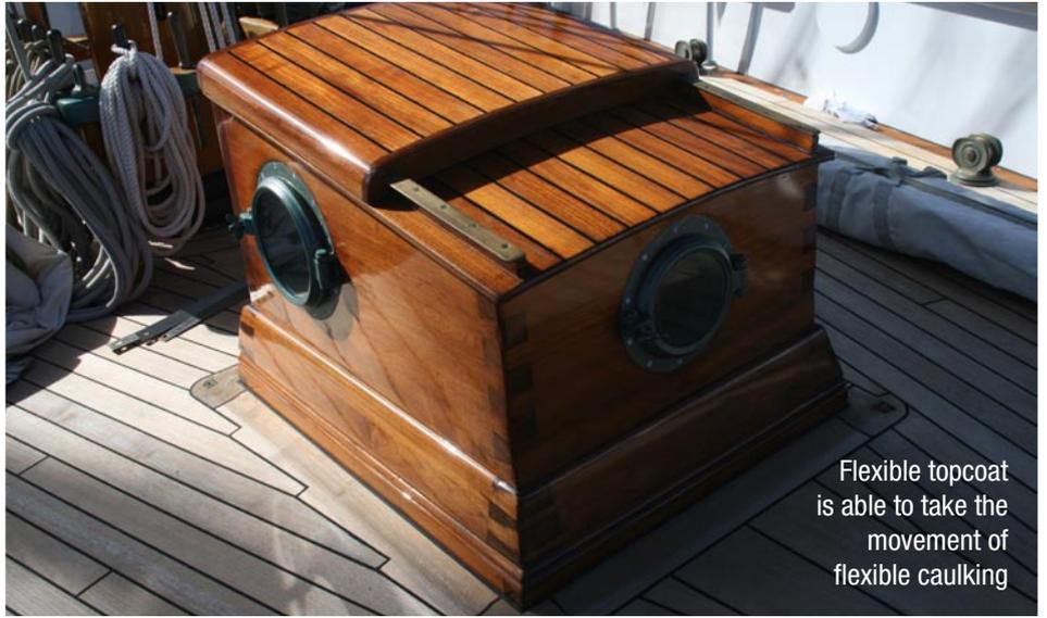
Flexible topcoat is able to take the movement of flexible caulking
